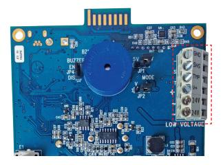
Three-conductor, 16 - 18 gauge wire / cable must be shielded when connecting to a remote analog transmitter. The LPT series remote analog transmitter enclosures have several conduit entry locations (general purpose enclosure). Under most local electrical codes, low voltage wires cannot not be run within the same conduit as line voltage wires.
