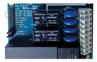
Place the second jumper on JP3 on either SET RLY ON DELAY or SET RLY OFF DELAY depending on the delay you wish to set. Once the jumpers are in position the test points TP1 and TP2 will output a voltage corresponding to the current time delay. The voltage is related to the delay using the following equation:
