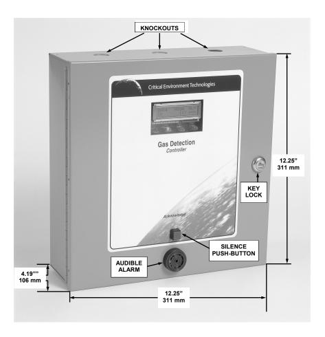
NOTE-1: Three knockouts can be found along the top edge and three along the bottom edge of the system enclosure
