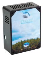
The YESDUST is a general purpose particulate sensor for use with a YES multi-channel monitor (e.g. YESAIR and YES Plus LGA). It operates from an internal rechargeable nickel hydride battery pack and connects to the auxiliary port of the YES multi-channel monitor with the supplied interface cable. The measured readings are displayed as another sensor on the LCD display of the YES multi-channel monitor, and are also data logged to the YES multi-channel monitor internal flash card, if utilized.
